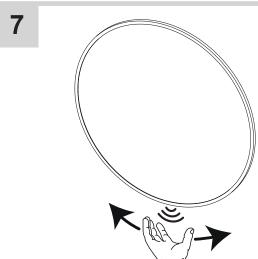
Your mirror comes with an infrared sensor located in the middle of the bottom. To activate the light and demisting pad, move your hand across the sensor once at a distance of around 5cm.
